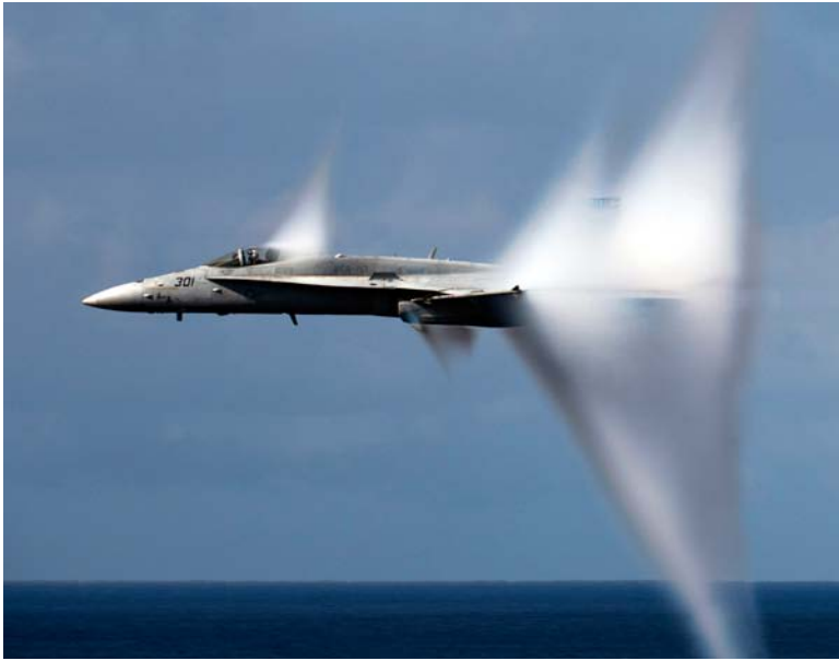
A U.S. Navy fighter jet breaks the sound barrier, causing water droplets to form clouds in the shape of shock waves.
